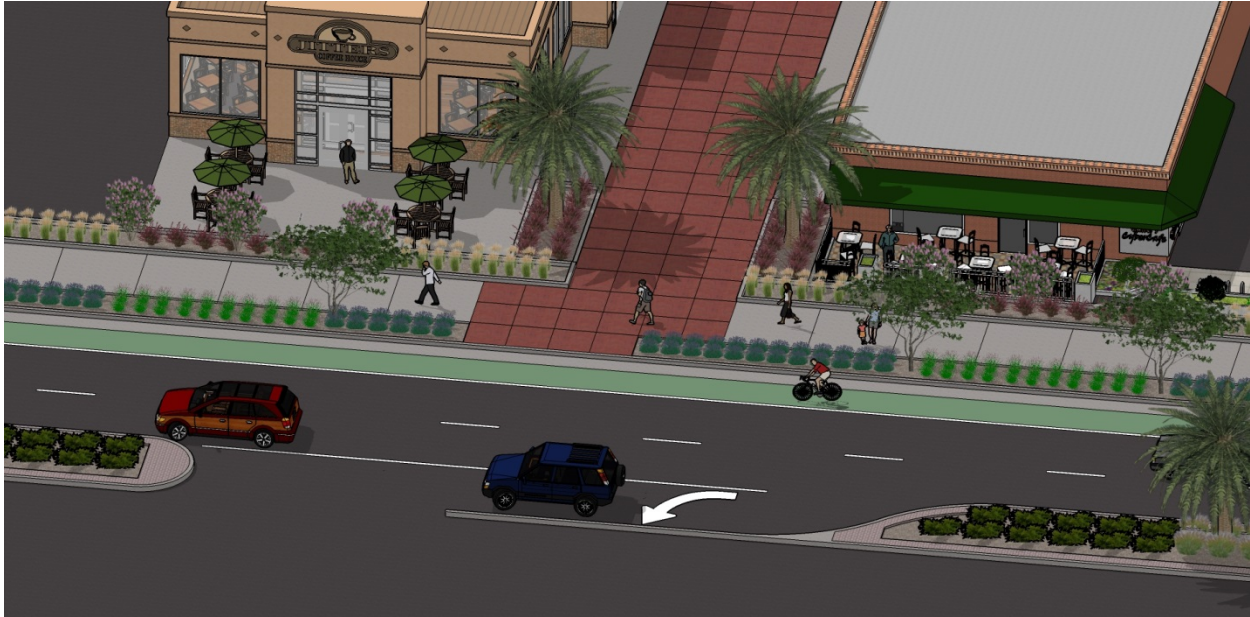
Figure 14 Proposed Streetscape Vision (Example shown with partial median and left-turn pocket access)
