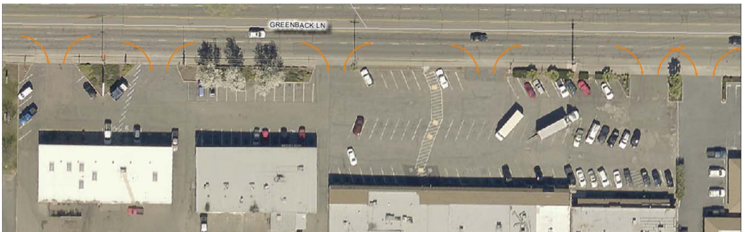
Figure 27 Redundant driveways in a short length of roadway
