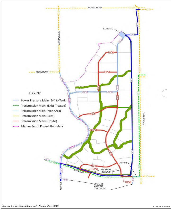
Plate PD-18: Proposed Trunk Domestic Water Delivery System Diagram
